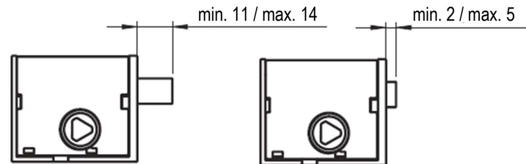
Modification with different pin length on request (in this case seal box will be removed)
